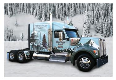
The new Kenworth W990 will transport the 2018 U.S. Capitol Christmas Tree from Oregon's Willamette Forest to Washington, D.C. The W990 is equipped with a 76-inch-mid-roof sleeper and the proprietary powertrain of PACCAR's MX-13 engine, 12-speed automated transmission, and 40K tandem rear axle. Central Oregon Truck Company in Redmond, Ore., was selected as this year's tour hauler. In commemoration of the Oregon Trail's 175th anniversary, the route will follow a reverse path of the famed trail.
