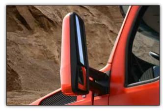
Durable aerodynamic side mirrors are cowl mounted for better stability and located farther forward and lower to optimize rearward visibility. The convex portion is 37 percent larger than Kenworth's standard convex mirror design.
