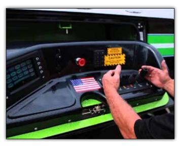
Configuration and control of your PTO functions has never been easier. User defined presets allow the engine and PTO to be set for optimal operation under any load. PTO controls are in the cab and can also be located remotely on the body and can operate up to two PTO's.
