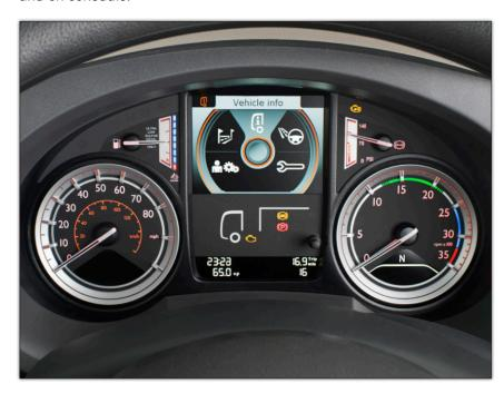
The dash has a familiar, contemporary design that presents critical driving information at a glance. An innovative 5 inch color master display module consolidates speed, engine RPM, oil level, fuel consumption, trip data, fault codes, outside air temperature, turbo pressure, PTO counter, service inspections and more. There is even an alarm clock.
