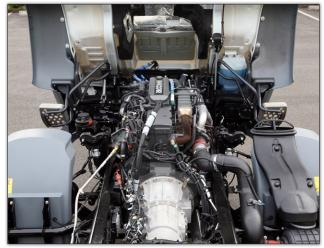
Standard equipment includes the proven, reliable and fuel efficient PACCAR PX-7 engine paired with an Allison 5 or 6-speed automatic transmission. You get plenty of power, acceleration and torque in a configuration that is a pleasure to drive.
